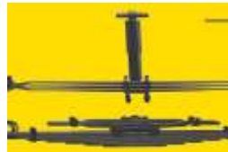
Lower NVH with improved engine mount and Parabolic suspension with rubber Bush
